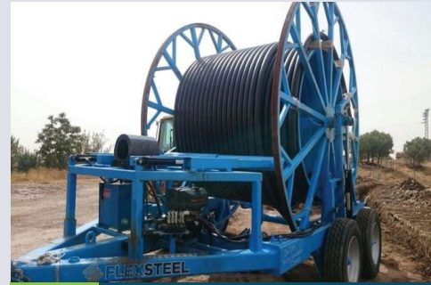
Fig.14: Flexsteel pipes on a trailer
